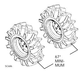
Figure 3. Tire Adjustment - 215 Loader Only
